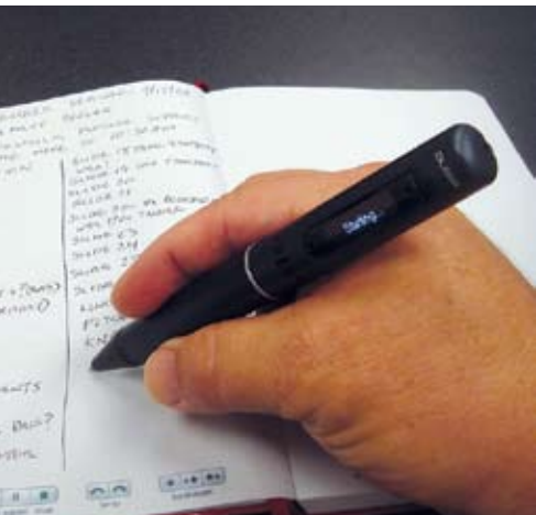
The Pulse pen synchronizes what is being said to the line of notes being made.
